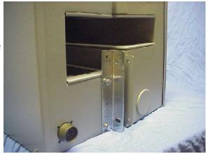
By mounting the brackets using the upper set of holes, the tunnel width is approximately doubled, allowing for more flexibility in what passes through the reader along with the code cards.
