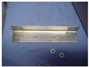
By mounting the brackets using the lower set of holes, the form factor of the new reader exactly matches the form factor of the original readers and can be used as an exact replacement.
